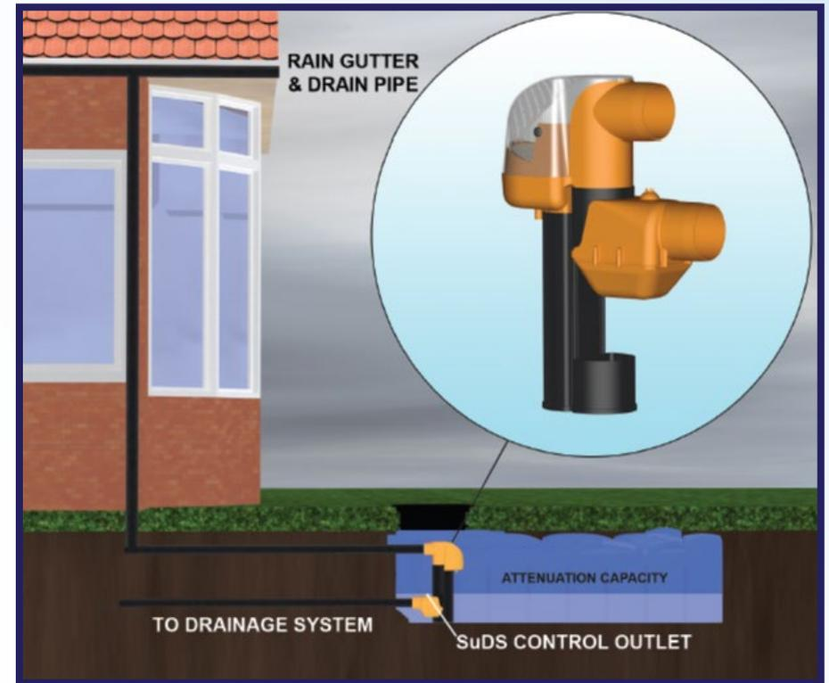
Every system we sell is bespoke, and calibrated to each site's requirements. Our engineers use Micro Drainage™ hydraulic modelling software to ensure the system discharges at the desired peak rate during a storm event.
